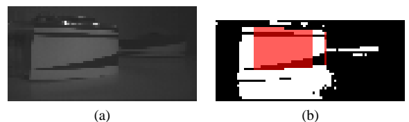
Figure 10. Body patten detection (a) Initial image. (b) the detected pattern is highlighted.
