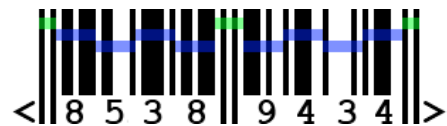
Figure 7. Structure of EAN-8 barcode, with the black-white-black pattern in the beginning, middle, and end.
