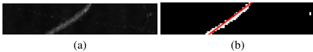
Figure 7: New introduced feature: (a) Initial image from a glowing trail received by e-puck camera. (b) Filtered image with a red directional line determined by Hough-Transformation (May, 2013)
